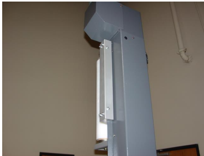
Film carriage at top of mast.
